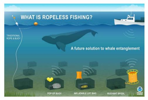
Ropeless gear for trap/pot fisheries with acoustic release devices is currently made by a variety of different companies and institutions. Some of those devices include:
