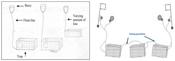
Fig. 1. Basic configuration of California commercial Dungeness crab, spiny lobster, and sablefish gear.<sup>6</sup>
