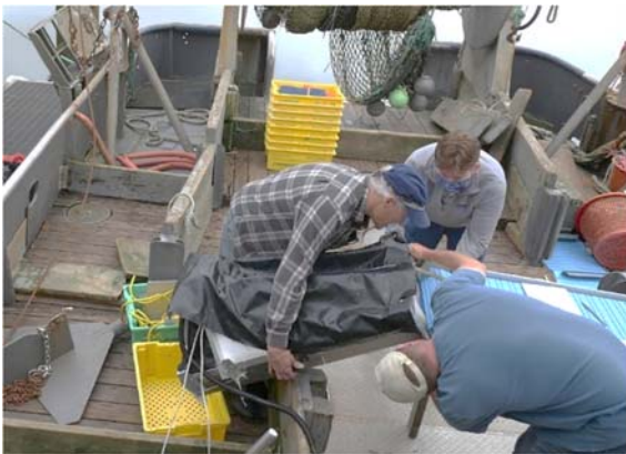
Figure 1 Installation of camera chute aboard the Cape Windy (photo credit Justin Smith)
